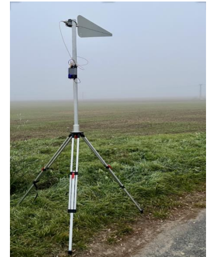
Omni- and directional antenna used by the spoofer
