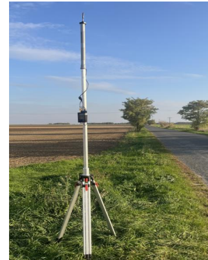
Omni- and directional antenna used by the spoofer
